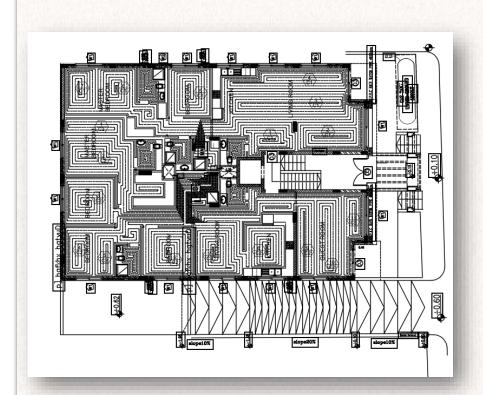
We offer a highly efficient underfloor heating system installed to the highest standards by the United Pioneering Business Company. Underfloor heating networks from the Italian emmeti system and emmeti pipes with an aluminum layer were used. Furthermore, emmeti pipes were used for the illuminator and the rest of the underfloor heating network's requirements for central lines. Heating controllers with wifi thermostat emmeti 2021-2022 were also used.
