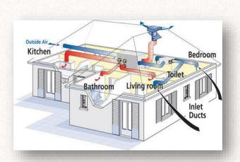
Mechanical ventilation enhances interior air quality by supplying fresh air and reducing pollutants, regulates moisture, avoids insufficient air movement, and eliminates the need for occupants to open windows.
